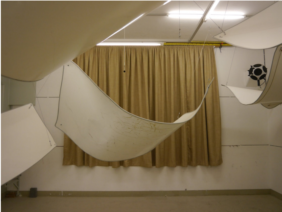
Figure B.1. Test arrangement in the reverberation room (frontal view).
